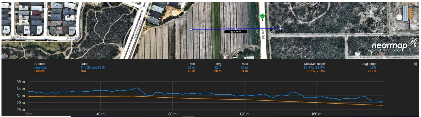
Figure 7. Slope across the land to the east (0.97°).
