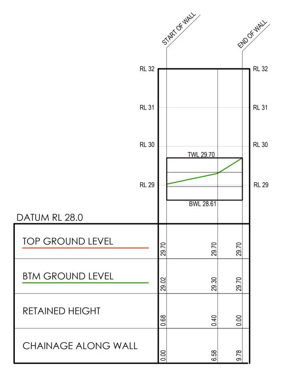
RETAINING WALL LONG SECTION (RET 4) SCALE 1:250 H 1:50 V
