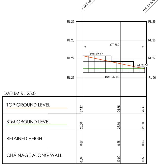
RETAINING WALL LONG SECTION (RET 3) - TWINSIDE WALL SCALE 1:250 H 1:50 V
